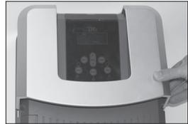
2. Remove the two screws which attach the lower cover to the main unit:
